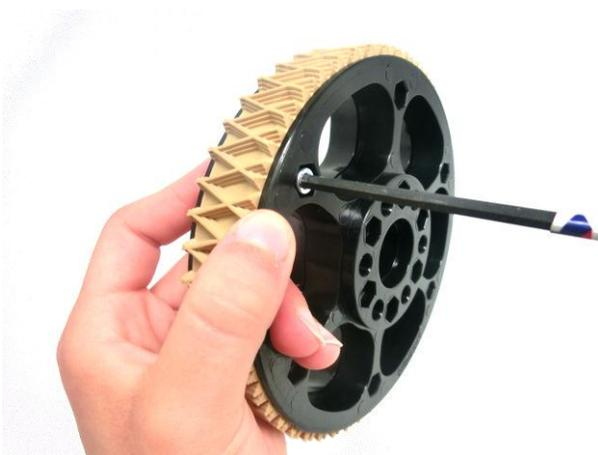
Step 5: Repeat step 4 until all the outer holes have a #10-32 Nylock Nut with its corresponding #10-32 x 1" SHCS.
